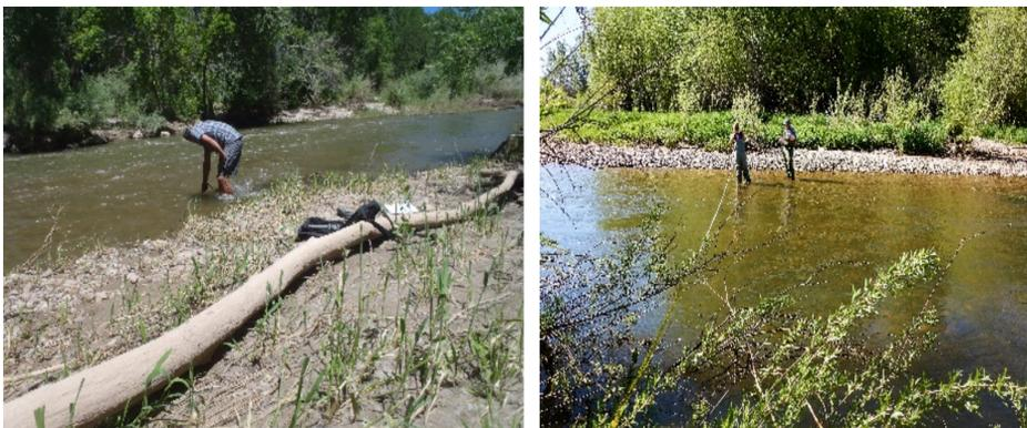
Figure 1: Measuring stream temperature, DO and TDS (left), and discharge (right)
